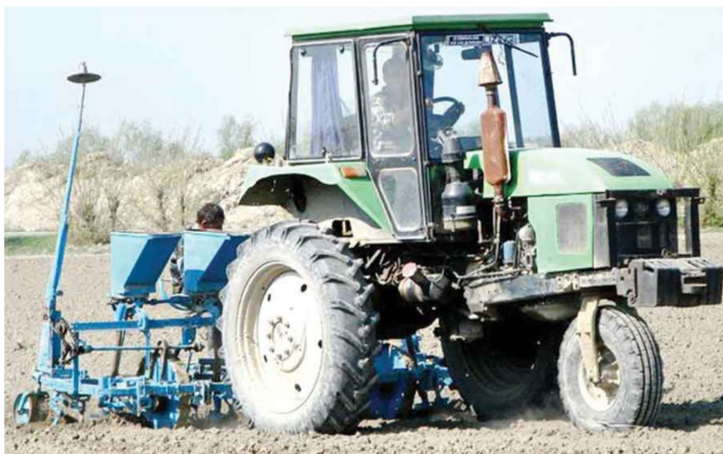
4.7-rasm. SCHX-3,6 chigit ekish agregati
