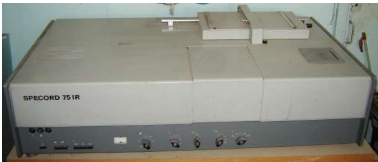
18.2-rasm. Spekord-75 spektrometrining ko‘rinishi (Germaniya).
