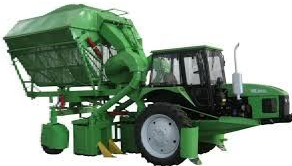
7-rasm. MX-1,8 rusumli paxta terish mashinasi
