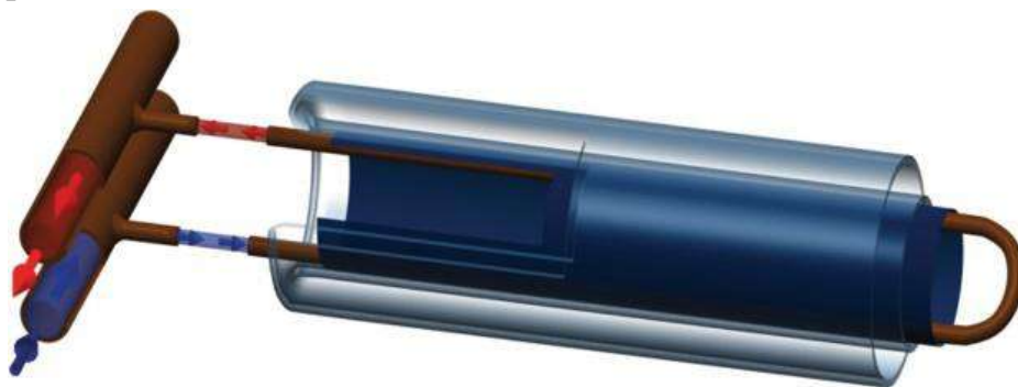
9-rasm. Silindrsimon absorber bilan to'g'ridan-to'g'ri isitishning U shaklidagi trubkasi
