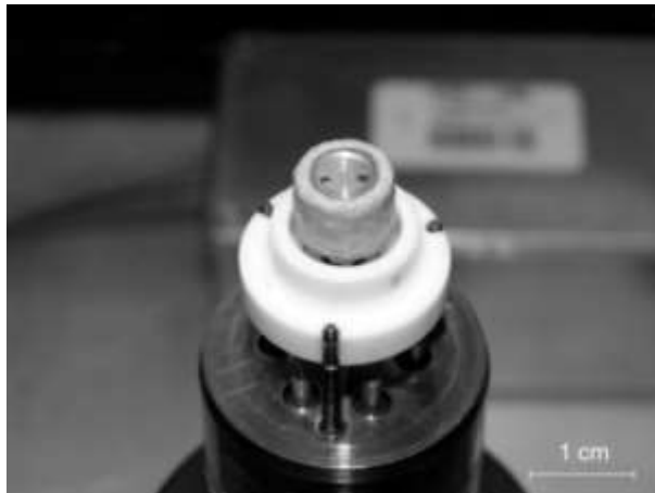
3.4-rasm. Yuqori bosimli DSC: Ichkarida namunali idish bilan kumush pech
