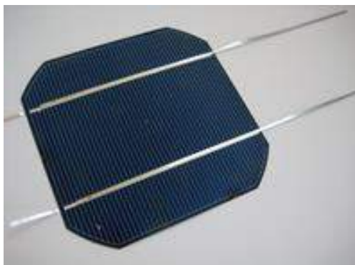
37-rasm. Yassi o‘tkazgich bilan payvandlangan QE (mis shinali o‘tkazgich)
