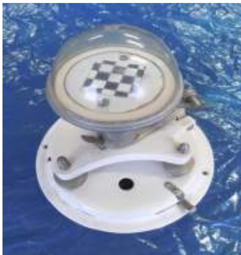
14-rasm. Universal piranometr M-80.
