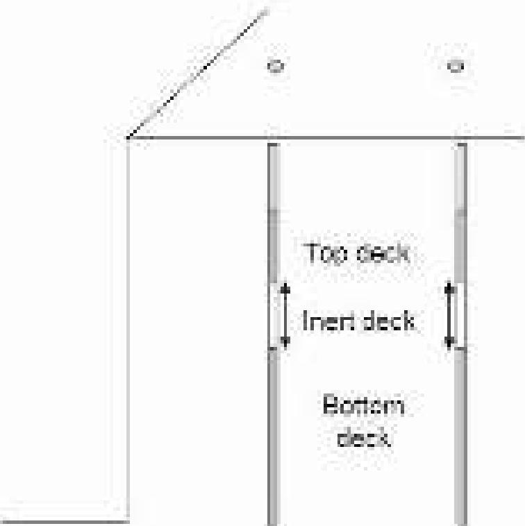
\*The minimum stemming between explosive decks should be six times the borehole diameter, and, in wet holes, this amount should be doubled.
