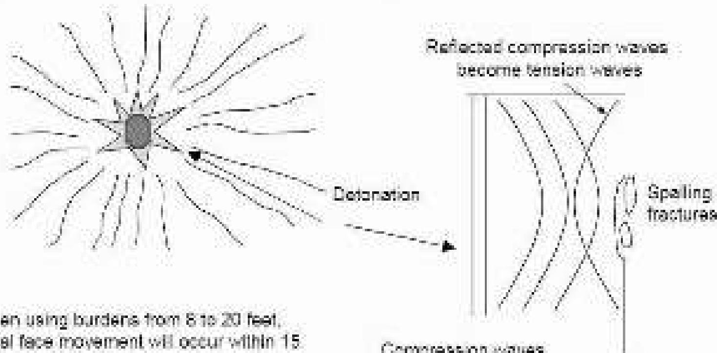
When using burdens from 8 to 20 feet, initial face movement will occur within 15 milliseconds. The crack network will establish and rock movement will begin after 1 millisecond per foot of burden on the hole.
