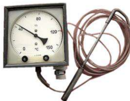
3.13-rasm. TKP-16SgV3T4 - portlashga qarshi himoyalangan, signal beruvchi kondensatsion termometr.
