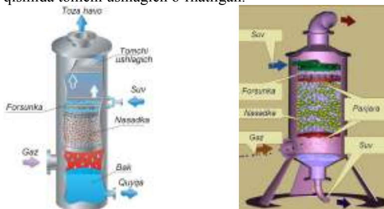
15.6-rasm. Mavhum qaynovchi nasadkali skrubber.
