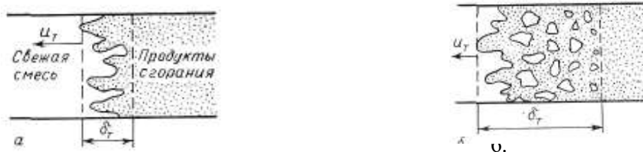
9.1-rasm. Aralashmaning turbulent yonishi: a - kuchsiz turbulent yonish; b - kuchli turbulent yonish.
