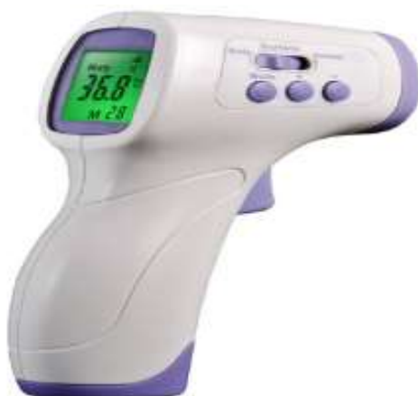
Infraqizil termometr yordamida haroratni o'lchash
