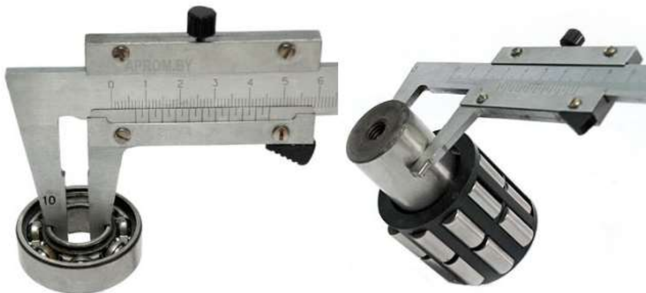
4.2– rasm. Podshipnik va uning o'lchamlari
