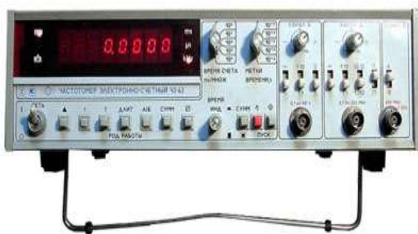
2.9 – rasm. Ch3-63 modelidagi chastotomer va uning metrologik tavsiflari
