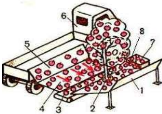
2-rasm. Meva yig'ish mashinasining (VUM-15A) tuzilishi va ish jarayoni: 1,4- ilgichlar; 2-tebratgich; 3-transporter; 5-ekran; 6-shassi; 7-konteyner; 8-ventilyator.
