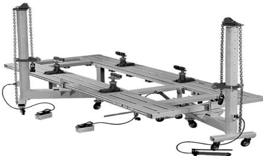
29-rasm. Yengil avtomobillar kuzovini tiklovchi "Siver S3-210" rusumli stend.
