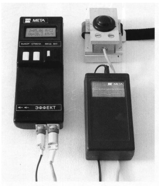
35-rasm. Tormoz tizimining samaradorligini aniqlovchi EFFEKT-02 jihoz.
