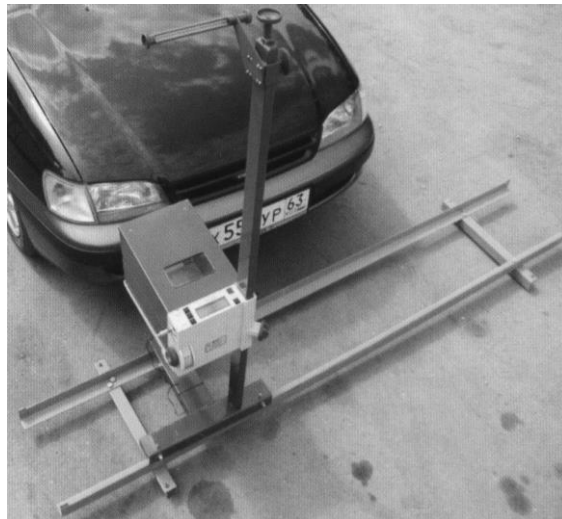
40-rasm. Avtomobil faralarining parametrlarini diagnos-tikalash uchun IPF-01 jihozi (a) va tekshirish jarayoni (b).
