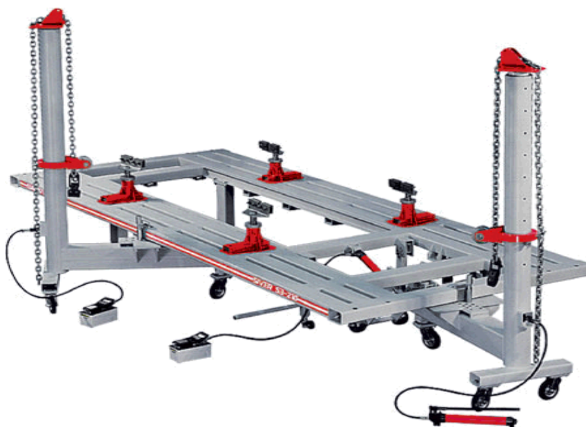
2.4-rasm. Yengil avtomobillar kuzovini tiklovchi Siver S3 210 rusumli stend.
