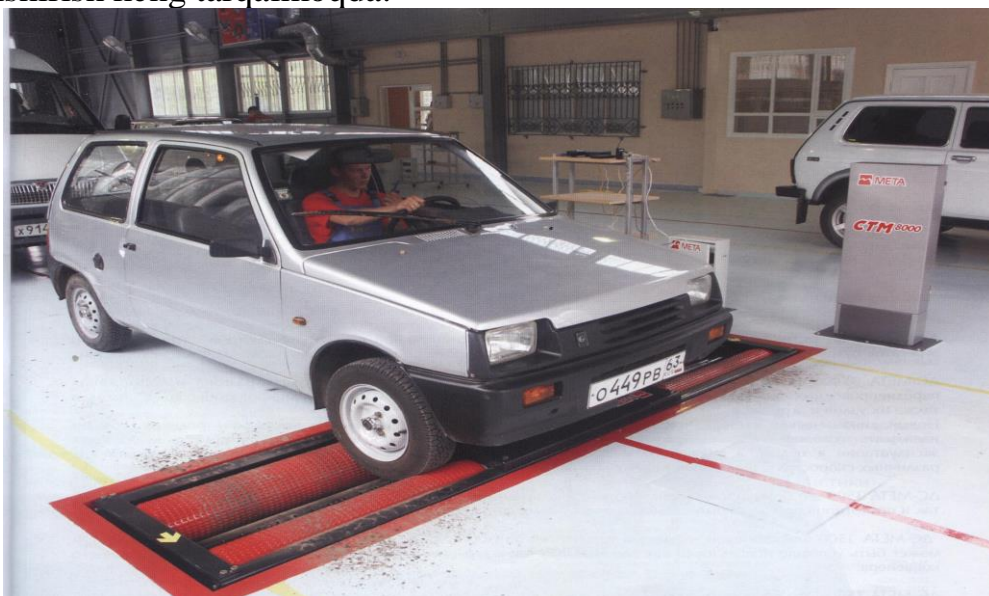
2.7-rasm. Rolikli STM-8000 rusmli stendda avtomobil tormozini diagnostikalash.
